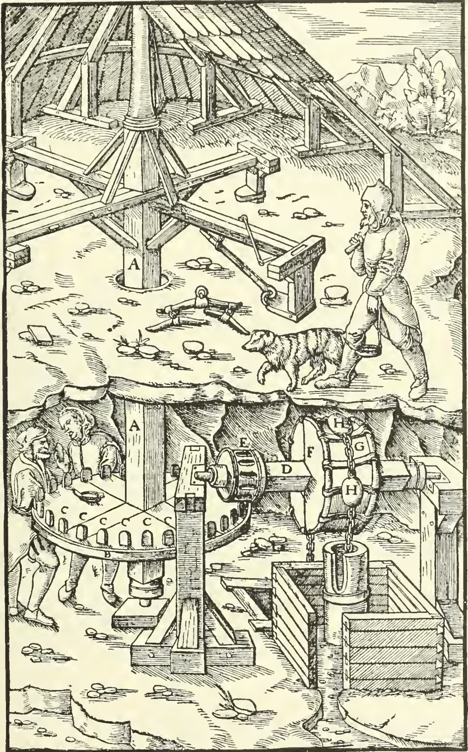
A—UPRIGHT AXLE. B—TOOTHED WHEEL. C—TEETH. D—HORIZONTAL AXLE. E—DRUM WHICH IS MADE OF RUNDLES. F—SECOND DRUM. G—DRAWING-CHAIN. H—THE BALLS.
